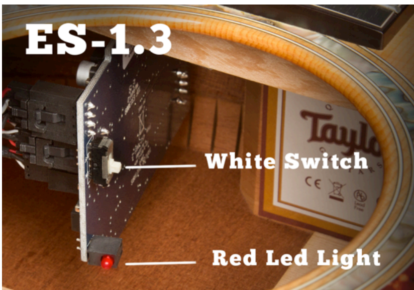
Image 1.6 Locating the red LED light & single white switch on an ES-1.3 preamp board
