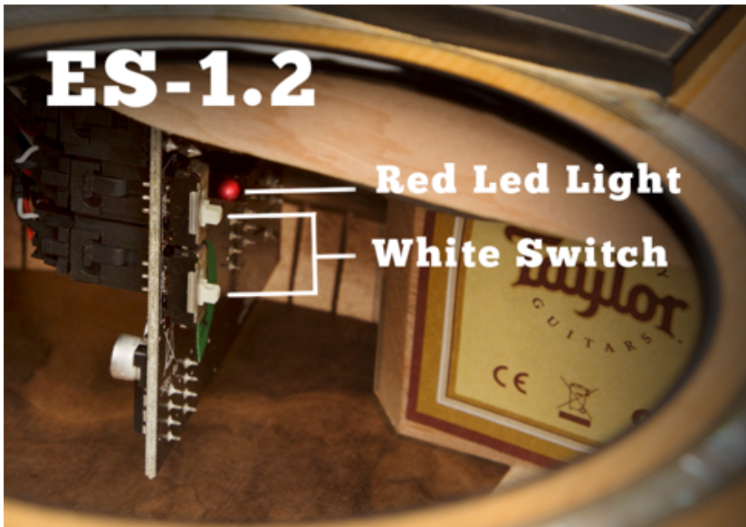
Image 1.7 Locating the red LED light & two white switches on an ES-1.2 preamp board
