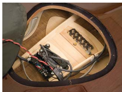
Inside the T5—the stacked humbucker and 12-string bridge plate are visible in the body cavity.
