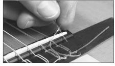
**14.** The slippery treble strings require a bit more care to keep them tight, but the technique is essentially the same. You can insert the string either way through the holes in the bridge. The high-E (treble) string has an additional loop to avoid slippage. Begin by looping the string under itself.
