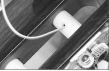
**6.** Pass the free end of the string toward the peghead, all the way through the tuner hole, from the top down, leaving a little slack. Make sure the top side of the tuner hole is pointed at a slight upward angle, toward the peghead.
