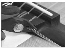
**18.** After tuning to pitch, snip the excess from the B and high-E strings.
