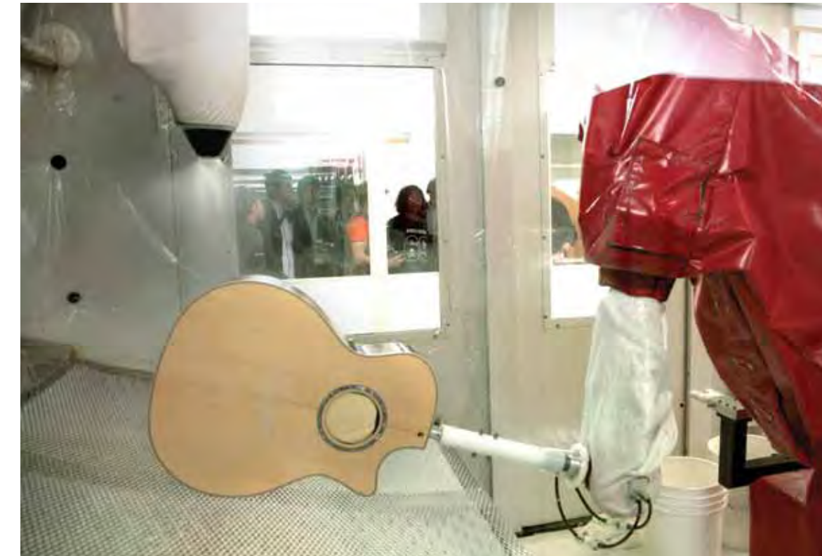
Opposite page (L-R): A road in Cameroon, where ebony is sourced; ebony fretboard blanks from Crelicam, a Cameroonian ebony mill now co-owned by Taylor; This page (from top down): Taylor's environmentally friendly polyester guitar finish is applied using a combined robotic/electrostatic spray system, which dramatically reduces material waste; a stack of milled mahogany for guitar necks
