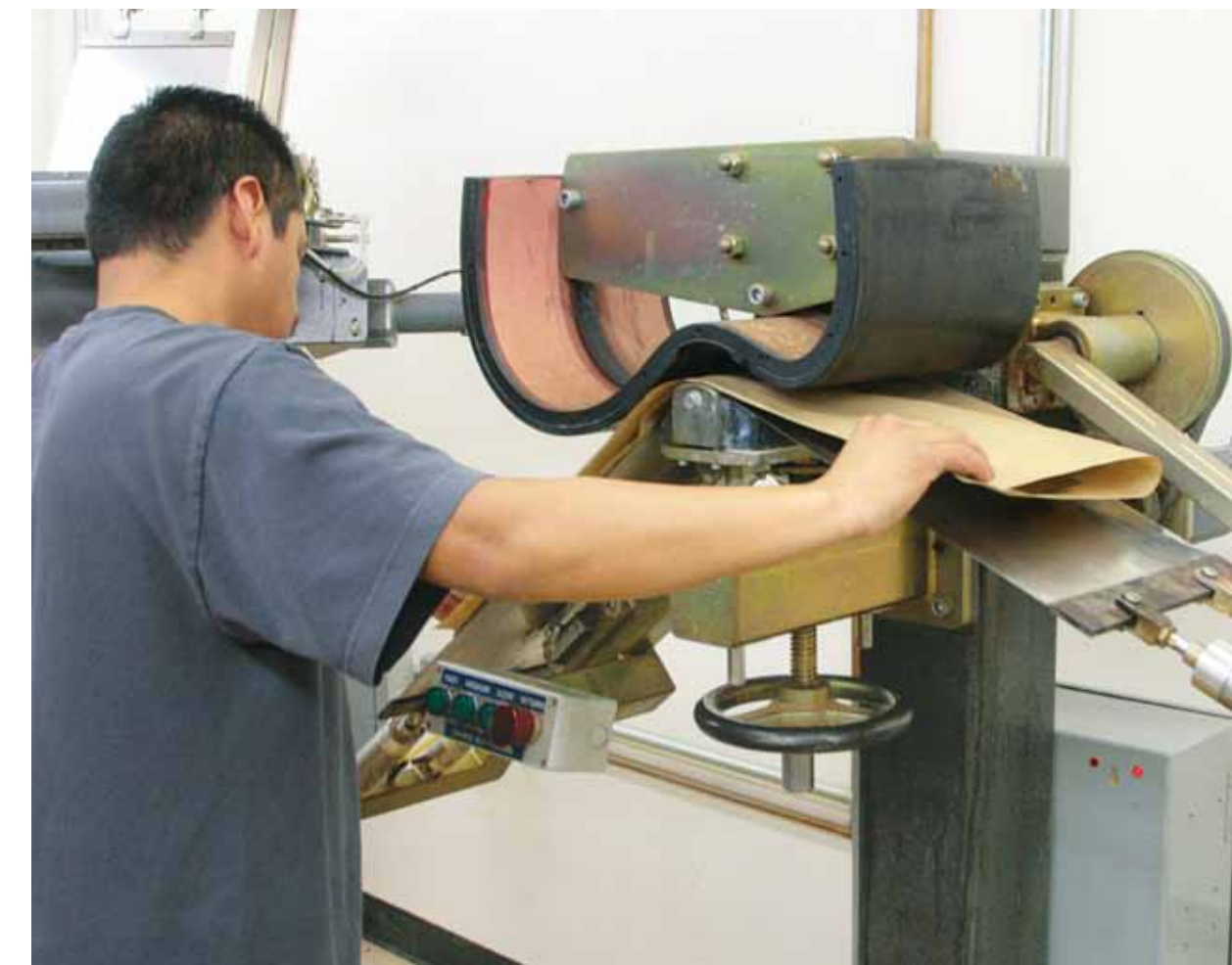
Opposite page: A computer-controlled mill brings precision and consistency to the neck-carving process; Above: Automated sidebending machines designed and built by Taylor's tooling department increase efficiency and reduce wood breakage
