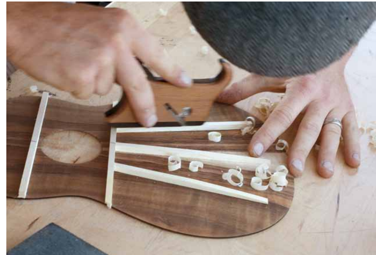
Andy Powers uses a rabbit plane to shave a ukulele's oversize braces down to begin the top voicing. "I'll work them slowly, going from one to the next until they all approach their finished size, monitoring the sound of the top as I go," he explains. "I made that plane on my 13th birthday, and have used it on nearly every guitar I've made since."
