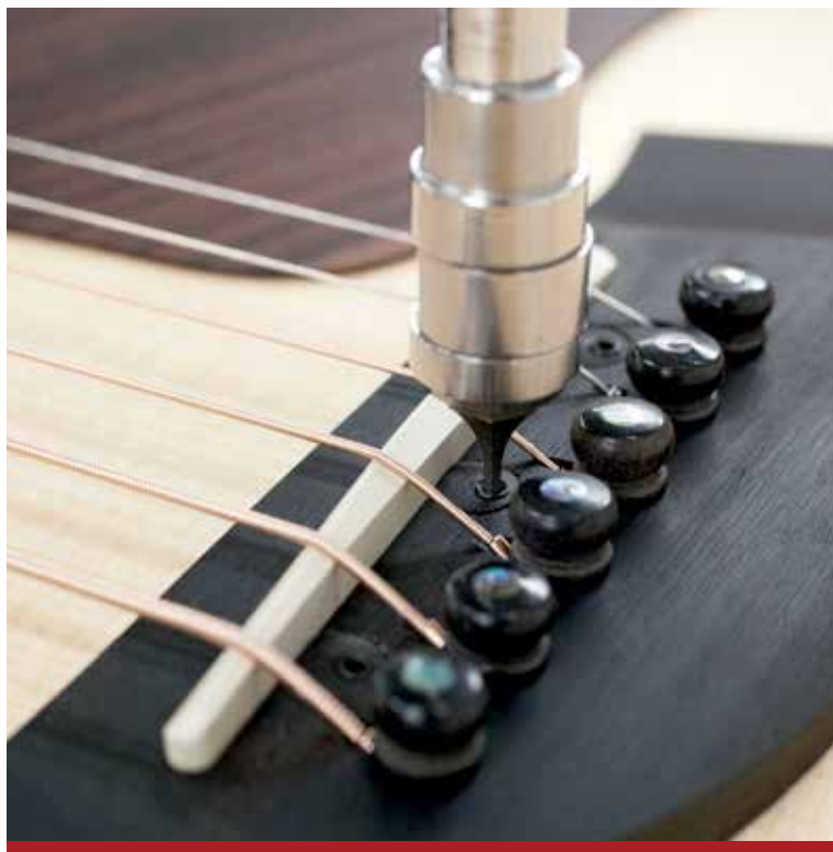
Three Allen screws enable proper calibration of each sensor's pressure against the saddle in Taylor's Final Assembly department. Once the pressures are factory set, no further adjustment should be required unless the saddle is being moved or replaced.
