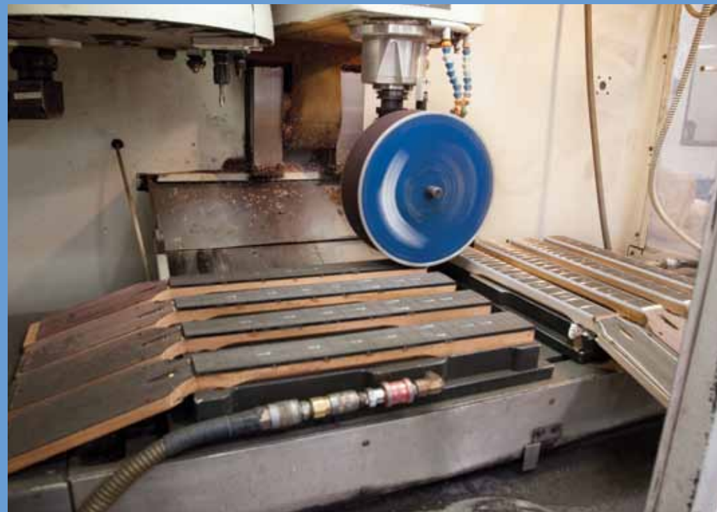
Below: A sampling of the guitar-making tools Guzzetta designed. L-R: A vacuum chuck, used to hold a guitar body without damaging the surface of the guitar while excess binding is scraped; a quick-change CNC sanding drum attachment, which enables the fretboard radius to be sanded; (opposite page) the fret buck, designed to absorb impact and protect the guitar when frets are hammered into the fretboard extension
