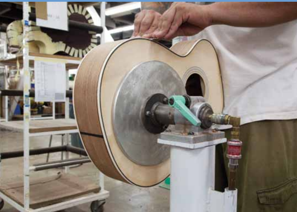
Below: A sampling of the guitar-making tools Guzzetta designed. L-R: A vacuum chuck, used to hold a guitar body without damaging the surface of the guitar while excess binding is scraped; a quick-change CNC sanding drum attachment, which enables the fretboard radius to be sanded; (opposite page) the fret buck, designed to absorb impact and protect the guitar when frets are hammered into the fretboard extension
