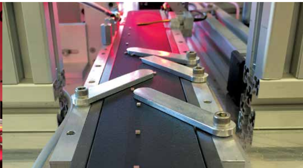
Piezo crystals travel into the workstation to be inspected by the vision system
