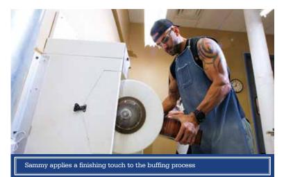
trying to pick something up, it'll stop," Tyler says. "Also, the buffing wheels can't run if the doors to the buffing cell are open. I like that a lot, especially because these wheels are lower to the ground, which would make it more dangerous if someone tripped."
